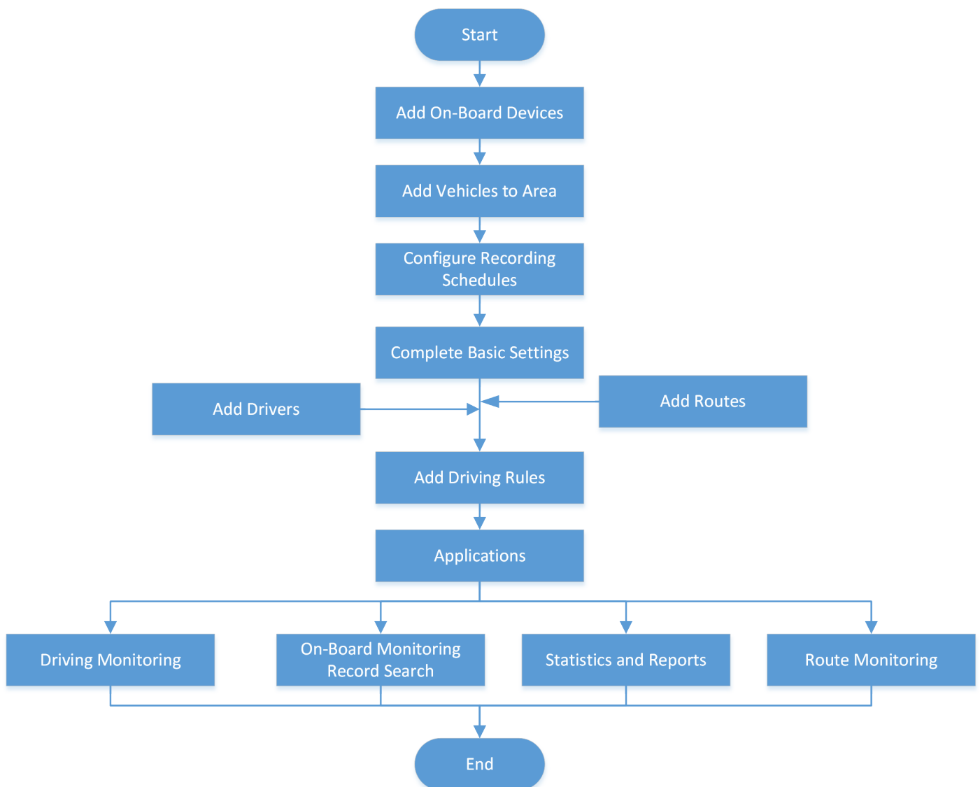
Figure 8-5 Flow Chart of On-Board Monitoring Configuration
